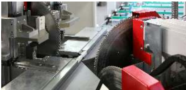
Fig.: Optima VI Saw unit with three saw blades
